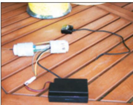
This shows the Byonics Micro-Trak 8000 installed in PVC tube with GPS and 12 V battery.
