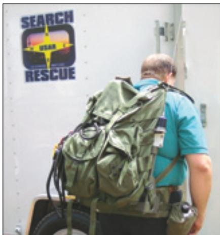
This shows a military style backpack (with metal frame) with a  $\frac{1}{2}$  wave mobile antenna installed. This solved the communication problem in the woods by extending the radio's transmission range about four times!
